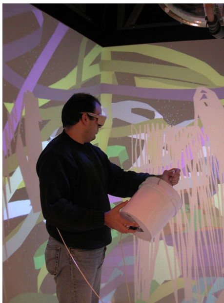
Figure 3.4: A physical bucket prop is used to throw virtual paint onto the walls and floor of the Cave.
